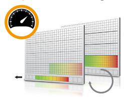
The active imaging area of the sensor is defined in a way that only a small section of the entire chip is used for imaging or spectral acquisition.
